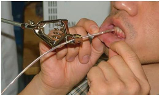
**Fig. 7** Prototype extra-oral imaging probe holder. To ensure reproducible re-imaging at exactly the same location during multiple imaging events and to minimize movement artifacts, a multi-joint imaging probe holder for OCT imaging was fabricated. In the future, this multi-joints holder can be replaced with a robotic arm for automatic programmed imaging localization (Figure Courtesy J.H.B.)
