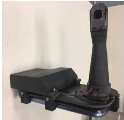
**Fig. 9** Smartphone snap-on oral cancer probe. (Courtesy P.W.S.)
